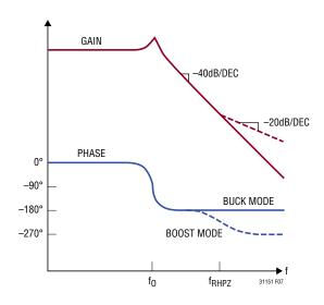
Figure 7. Buck-Boost Converter Bode Plot
