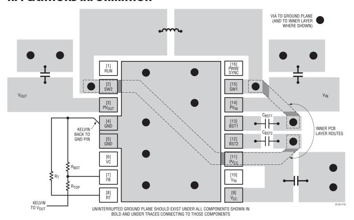
Figure 15. PCB Layout Recommended for the DHD Package
