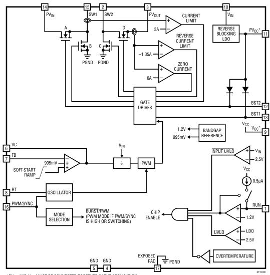
\*PV $_{CC}$  and v $_{CC}$  must be connected together in the application the exposed pad is an electrical connection and must be soldered to the board and electrically connected to ground
