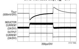
1.5A Load Step,  $V_{IN} = 10.6V$
