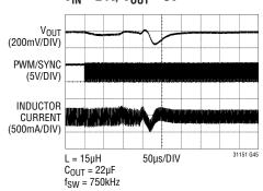
Phase-Locked Loop Release,  $V_{IN} = 24V$ ,  $V_{OUT} = 5V$
