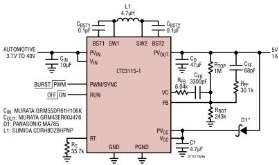
\*OPTIONAL-INSTALL D1 FOR IMPROVED EFFICIENCY AND LOWER INPUT OPERATING VOLTAGE
