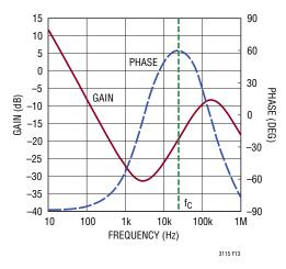
Figure 13. Compensated Error Amplifier Bode Plot
