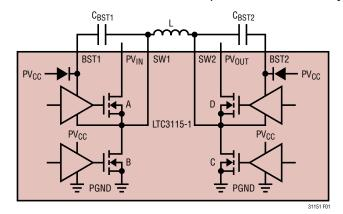
Figure 1. Power Stage Schematic
