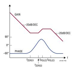
Figure 10. Type III Compensation Bode Plot
