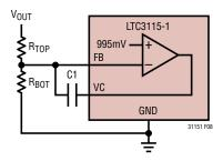
Figure 8. Error Amplifier with Type I Compensation
