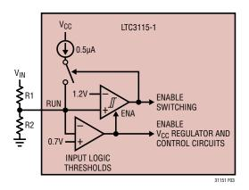
Figure 3. Accurate RUN Pin Comparator
