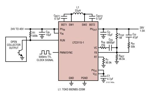
**Output Voltage from Noisy Input Rail**
