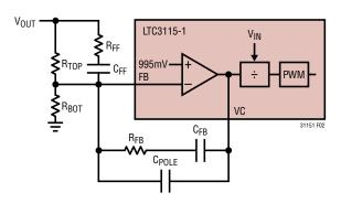
Figure 2. Error Amplifier and Compensation Network
