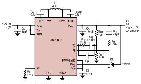
C<sub>IN</sub>: MURATA GRM55DRG1H106K C<sub>O</sub>: OS-CON 105VPA150MAA D1: PANASONIC MA785 L1: COILCRAFT MSS1260
