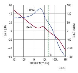
Figure 14. Complete Loop Bode Plot
